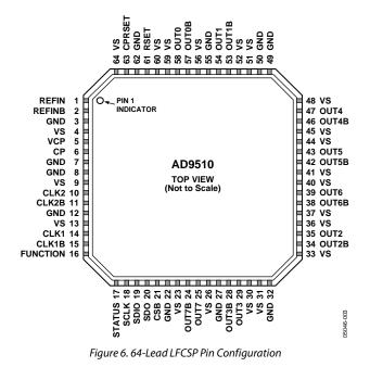
Note that the exposed paddle on this package is an electrical connection as well as a thermal enhancement. For the device to function properly, the paddle must be attached to ground, GND.
