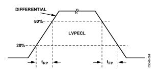
Figure 3. LVPECL Timing, Differential
