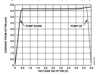
Figure 17. Charge Pump Output Characteristics @ VCPs = 5.0 V
