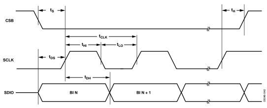
*Figure 51. Serial Control Port Timing—Write*
