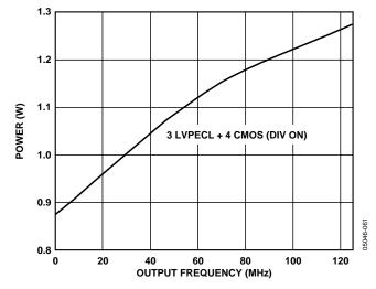
Figure 10. Power vs. Frequency—LVPECL, CMOS (PLL Off)
