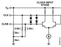
Figure 35. CLK1, CLK2 Equivalent Input Circuit
