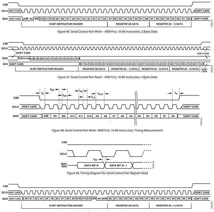
Figure 50. Serial Control Port Write—LSB First, 16-Bit Instruction, 2 Bytes Data
