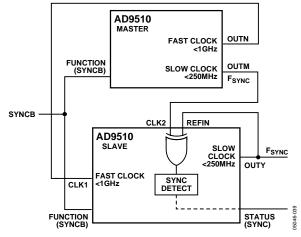
Figure 43. Multichip Synchronization
