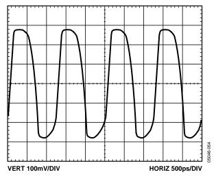
Figure 19. LVDS Differential Output @ 800 MHz
