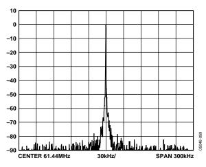
Figure 15. Phase Noise, LVPECL, DIV 4, FVCXO = 245.76 MHz, FOUT = 61.44 MHz, FPFD = 1.2288 MHz, R = 25, N = 200
