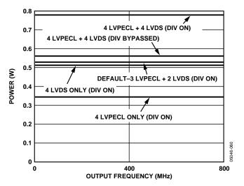
Figure 7. Power vs. Frequency—LVPECL, LVDS (PLL Off)
