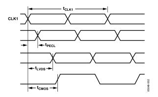
Figure 2. CLK1/CLK1B to Clock Output Timing, DIV = 1 Mode
