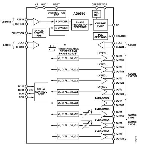
Figure 33. Functional Block Diagram Showing Maximum Frequencies
