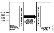
Figure 45. Relationship Between Serial Control Port Register Buffers and Control Registers of the AD9510
