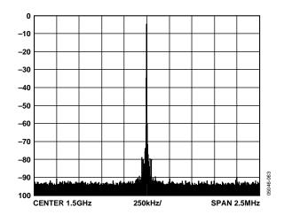
Figure 13. PLL Reference Spurs: VCO 1.5 GHz, FPFD = 1 MHz
