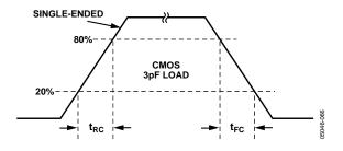
Figure 5. CMOS Timing, Single-Ended, 3 pF Load
