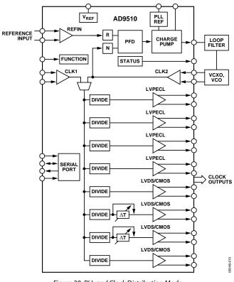
Figure 30. PLL and Clock Distribution Mode
