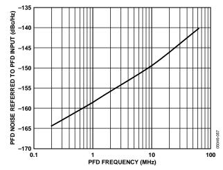
Figure 16. Phase Noise (Referred to CP Output) vs. PFD Frequency
