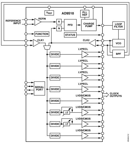
Figure 32. AD9510 with VCO and BPF Filter
