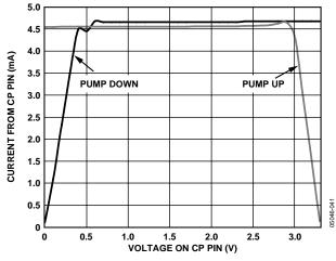
Figure 14. Charge Pump Output Characteristics @ VCPs = 3.3 V
