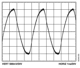
Figure 20. CMOS Single-Ended Output @ 250 MHz with 10 pF Load
