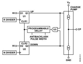
Figure 36. PFD Simplified Schematic and Timing (In Lock)
