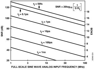
Figure 53. ENOB and SNR vs. Analog Input Frequency
