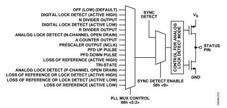
Figure 37. STATUS Pin Circuit CLK1 Clock Input
