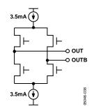
Figure 42. LVDS Output Simplified Equivalent Circuit
