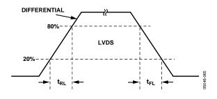
Figure 4. LVDS Timing, Differential
