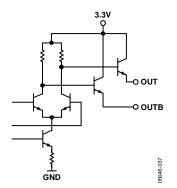
Figure 41. LVPECL Output Simplified Equivalent Circuit
