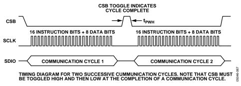
Figure 52. Use of CSB to Define Communications Cycle
